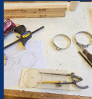
I assembled all the pieces, with masking tape to hold them together, and spread glue on the edges between each staff. Use cheap brushes with glue!
