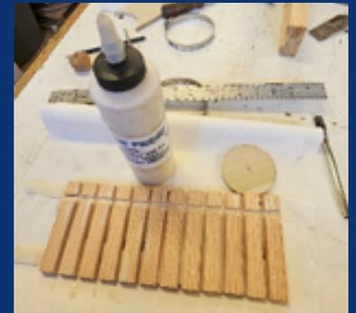
To get a really tight fit for gluing, I use hose clamps. Rubber bands also work well.
